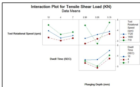
FIGURE 6. Interaction plots for tensile-shear load.
