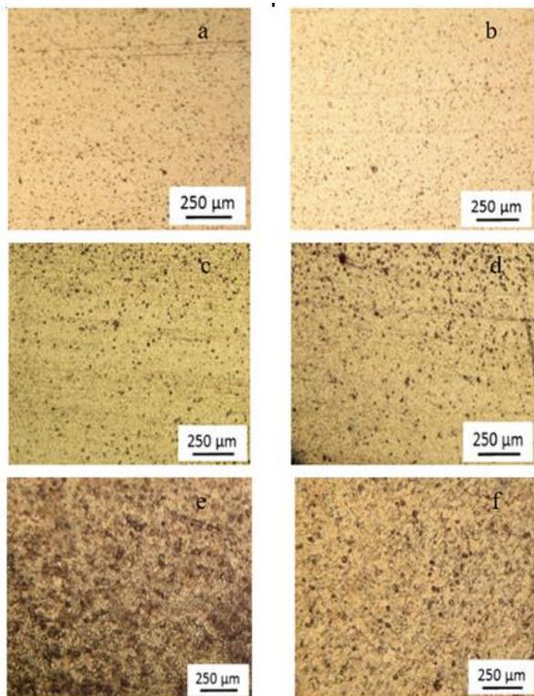
**FIGURE 4.** Microstructure of at the stirred zone of samples FSSWed at: (a,b) 710 rpm, 4 sec., 3.05 mm, (c,d) 710 rpm, 10 sec., 3.15 mm, and (e,f) 1120 rpm, 7 sec., 3.05 mm.
