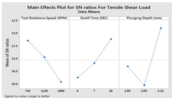
FIGURE 5. Main effects plot for tensile-shear load.
