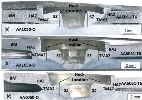
**FIGURE 3.** The macro cross-section views of friction stir spot joints FSSWed at (a) 710 rpm, 4 sec., 3.05 mm, (b) 710 rpm, 10 sec., 3.15 mm, and (c) 1120 rpm, 7 sec., 3.05 mm.
