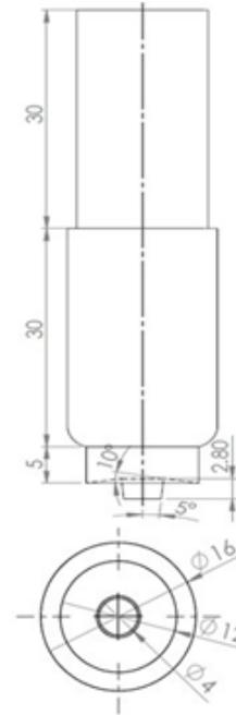
**FIGURE 2.** Schematic illustration of the tool used in the present study (dimensions in mm).
